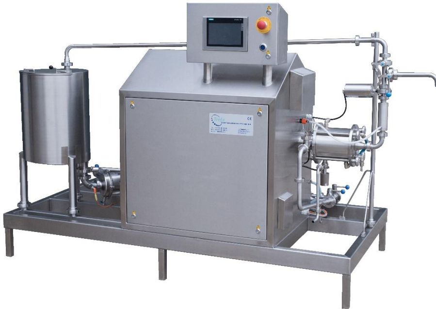
Trefa machine with buffer tank and CIP unit built on one frame.
